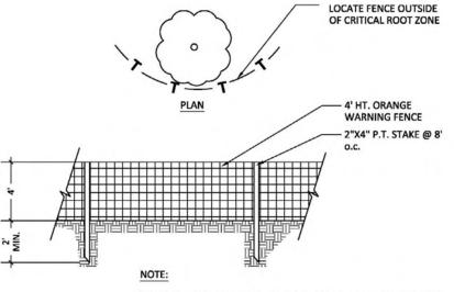
PROVIDE FENCE AS SHOWN ON PLAN. PROVIDE AT LEAST ONE FOOT OF DISTANCE FROM TREE TO FENCE FOR EACH INCH OF TREE DBH, WHERE DBH REFERS TO THE TREE DIAMETER MEASURED AT 4.5' ABOVE THE GROUND.
